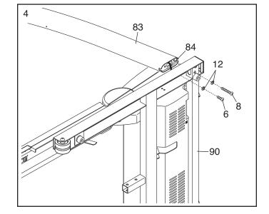
5. With the help of a second person, carefully tip the treadmill onto its right side. Partially fold the Frame (51) so the treadmill is more stable; **do not fully fold the Frame yet.**
